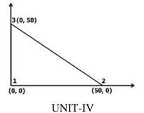
7. Find the Jacobian determinant [J] of the two dimensional element at  $\xi=0$  and [12M]  $\eta=0$  as shown in figure.
